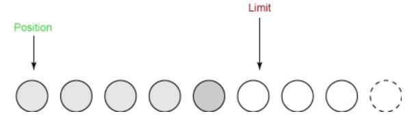
We are now ready to begin writing data to a channel from the buffer. The position has been set to 0, which means the next byte we get will be the first one. And the limit has been set to the old position, which means that it just includes all the bytes we read before, and no more.
