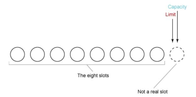
The position is set to 0. If we read some data into the buffer, the next byte read will go into slot 0. If we write from the buffer, the next byte taken from the buffer will be taken from slot 0. The position setting is shown here:
