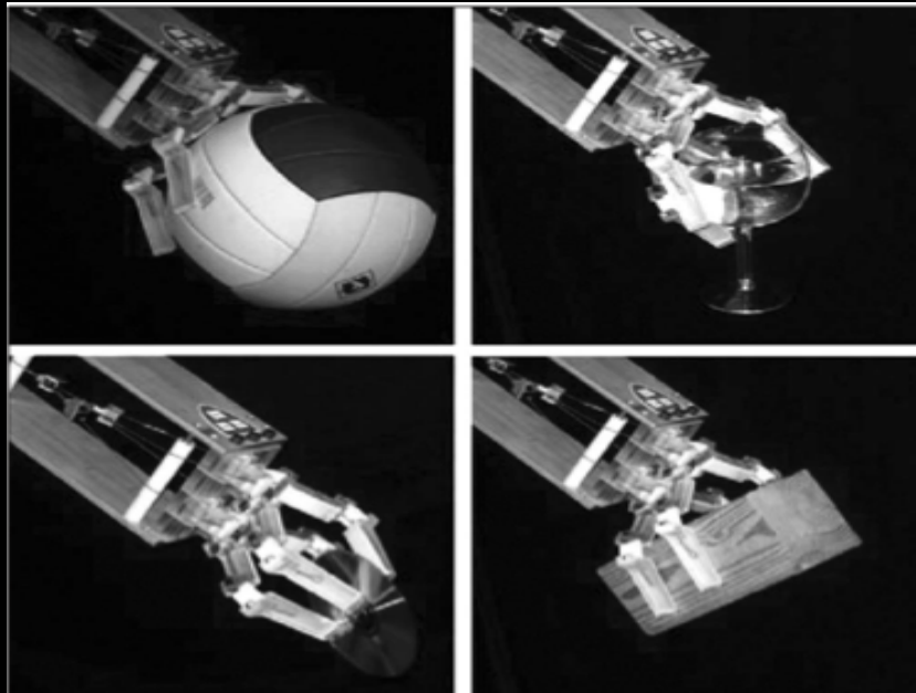
Figure 12. A compliant grasper developed by A. Dollar and R. Howe at Harvard University leverages its adaptive physical design to robustly grasp unknown objects [16].
