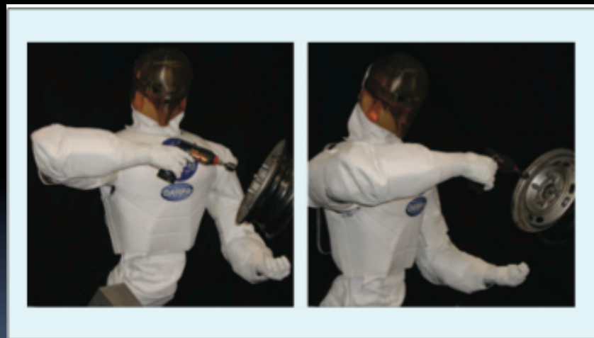
Figure 6. Researchers from Brown and Vanderbilt have been developing methods that enable Robonaut to learn to behave autonomously from teleoperated examples. At the workshop, they presented a method that discovers instances of success and failure from teleoperated examples of Robonaut using a power drill [11].
