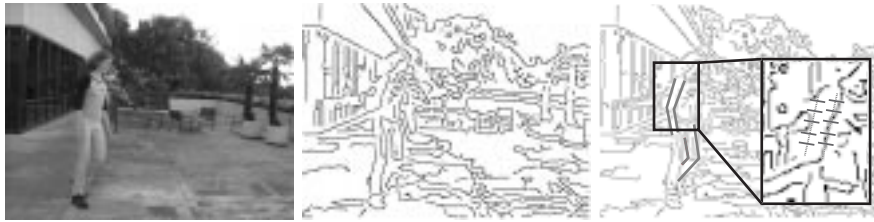
Figure 3. Example of edge detection using the Canny filter. Left: Original image. Center: Typical Canny edges; too many edges in some regions, too few in others. Right: How should predicted limb edges be compared with the detected edge locations?
