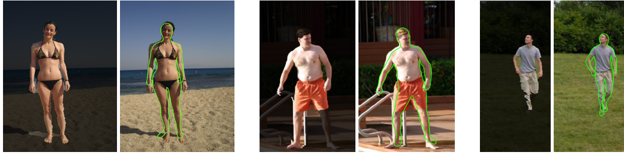
Figure 8. Comparison to GrabCut. GrabCut with a manual initialization step and no manual cleanup, compared to fully automatic CP segmentation.
