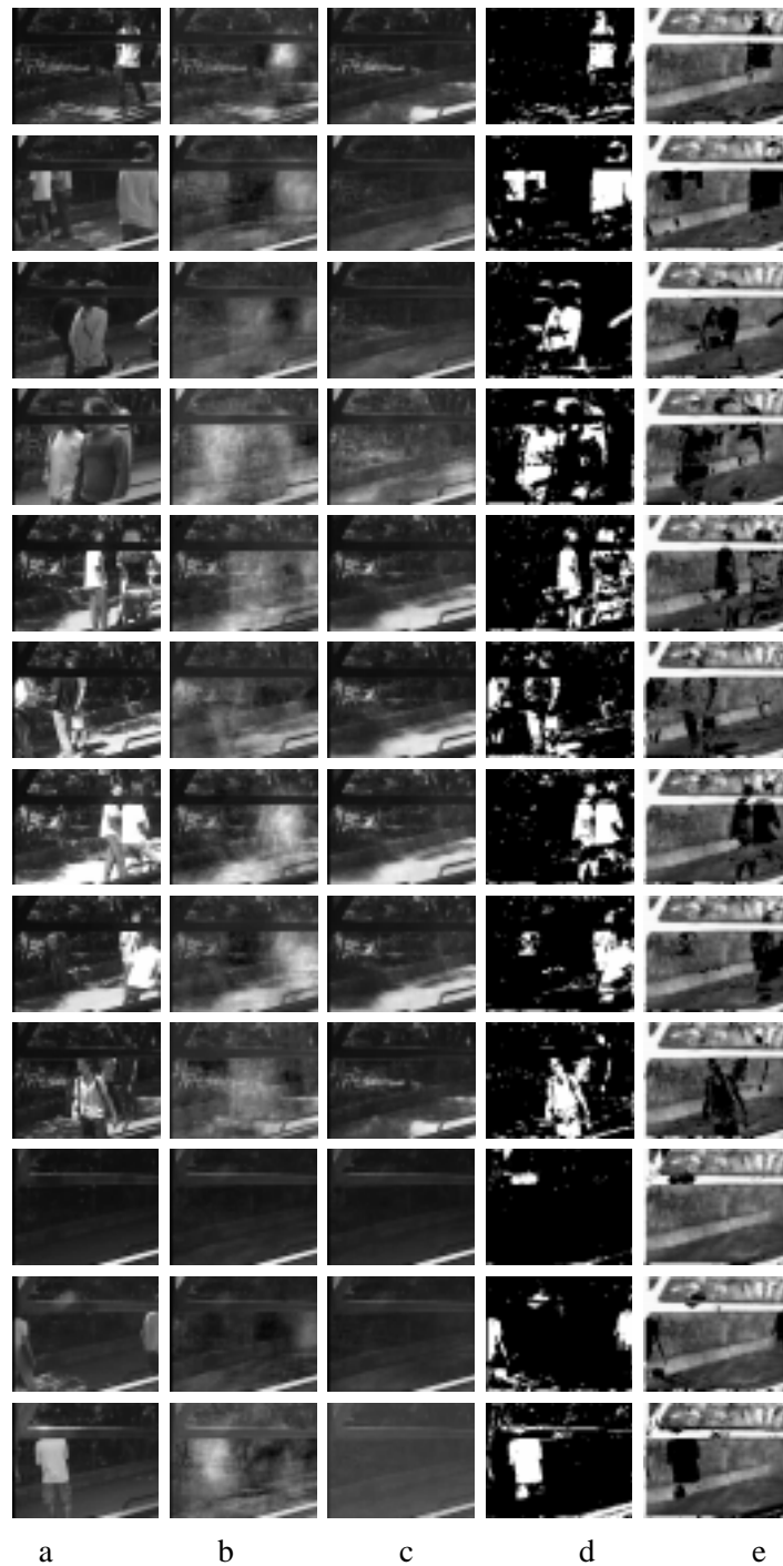
Figure 12: (a) Original Data. (b) PCA reconstruction. (c) RPCA reconstruction. (d) Outliers. (e) Weights.
