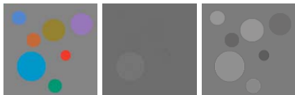
Figure 4: Converting the source image (Left) to grayscale with Photoshop’s grayscale mode results in a nearly featureless image (Middle). The Color2Gray algorithm creates circles that are distinct from the background (Right). Parameters: \theta = 180^\circ ; \alpha = 8 ; \mu = entire image.
