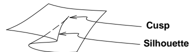
Figure 7: A cusp occurs at the end of a silhouette. A slight “hook” is conventionally drawn at the cusp to indicate its shape.
