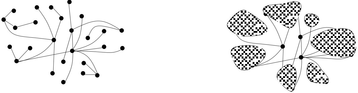
Figure 3: The figure on the left shows an arbitrary spanning tree T^* for the same input graph G . The figure on the right has r shaded regions, one for each subset V_i of nodes corresponding to a tree T_i in Figure 3.2. The proof of the algorithm's performance guarantee is based on the observation that at least r + |S| - 1 edges are needed to connect up the V_i 's and the nodes in S .
