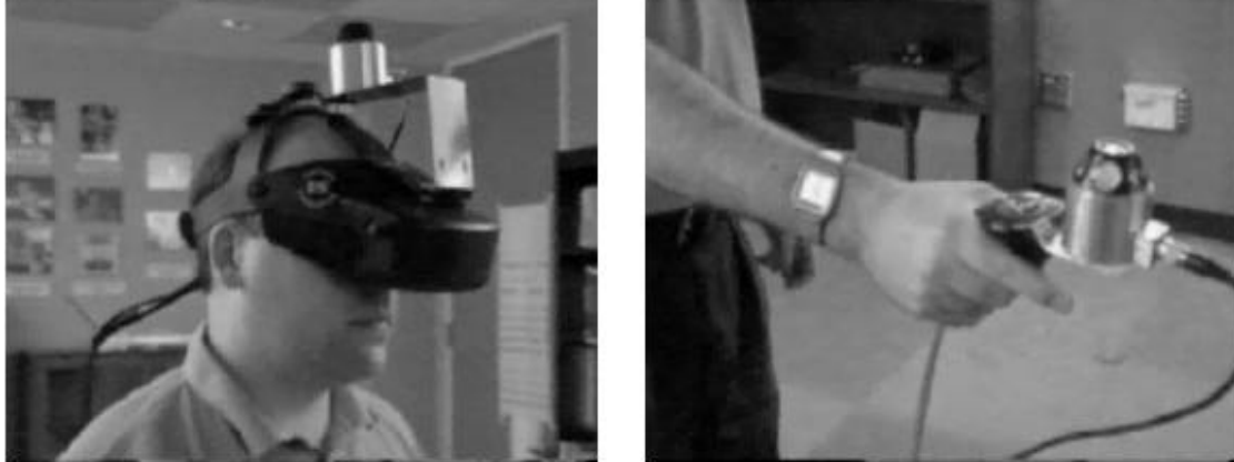
Figure 2.6 HiBall HiBall is used as a head tracker or a 3D digitization probe: A pencil-shaped fibreglass wand is linked to the end of a HiBall
