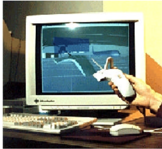
Figure 2.12 Virtual Tricorder Interface The user is using a virtual tricorder to select items from a virtual menu. The physical prop and the virtual tricorder have a familiar transition which reduces the user's cognitive load.
