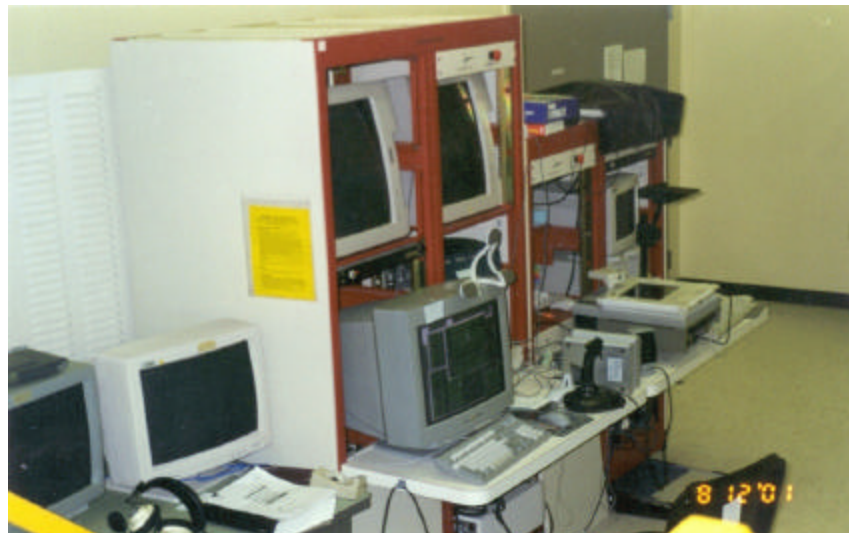
Figure 3.5 Instructor / Operator Working Area The operator monitors the subject's view by observing the upper two monitors which display the same images as the two Triuniplex projectors inside the dome, one for each eye. The lower monitor outputs from the SGI Octane
